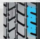
The semi-closed shoulder design helps prevent uneven shoulder wear.
